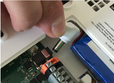
Plug in the power connector
