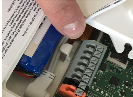
Route the wire behind the retainer clip
